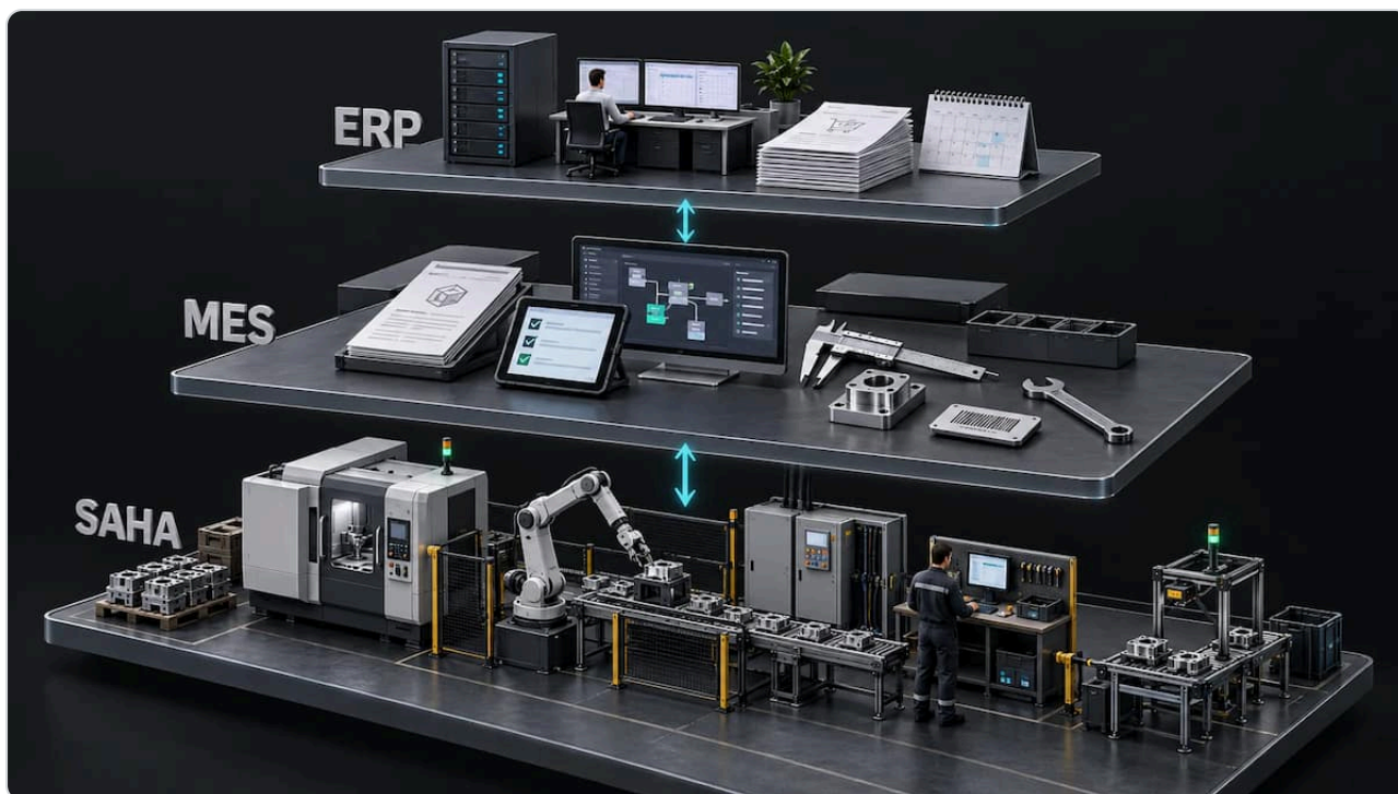
Figure 1. Simplified functional relationship: ERP passes down the plan, MES executes production and feeds back actual results. The image is not a network security topology.
