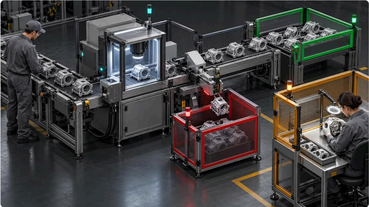
Figure 2. At a quality wall, conforming, nonconforming and undecided outcomes must be managed physically. The colors only support the illustration; they do not replace identity and authorization controls on the shop floor.
