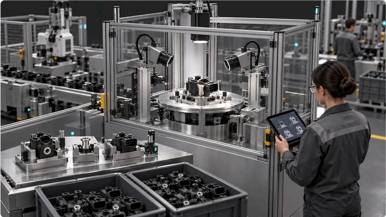
Figure 3. Multiple images increase coverage of visible surfaces. Cameras do not, on their own, take over function, torque or leak tests.
